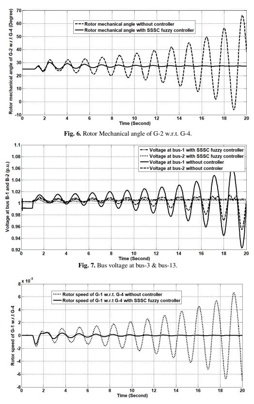
Fig. 8. Rotor speed deviation of G-1 w.r.t. G-4.
