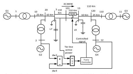
Fig. 3. Two-area four-machine interconnected power system with a SSSC installed in series with the transmission line.
