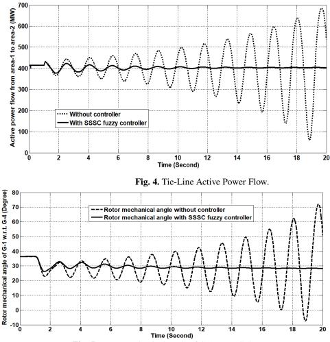
Fig. 5. Rotor Mechanical angle of G-1 w.r.t. G-4.
